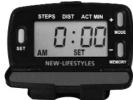
1. Press the **+** button until the flashing digit reflects the correct hour. Use the **-** button to back up, if needed. Pay attention to the AM or PM below the hour to set the correct time.
